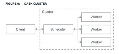
The cluster is composed of a *scheduler*, which is responsible for distributing the calculation tasks among the different available *workers*. Those workers can have an arbitrary number of CPU cores and GPUs depending on the hardware used and how Dask is set up.
